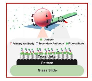
**Figure**: Schematic of MBL for patterning living matter – first an organic substrate is patterned on a glass cover-slip, followed by a cross-linker to enhance adhesivity of the biomolecules, after which biomolecules in the form of a primary antibody, and then a secondary antibody/antigen tagged with fluorophores is patterned. Fluorescence is observed on laser illumination, demonstrating the retention of activity of the species patterned.
