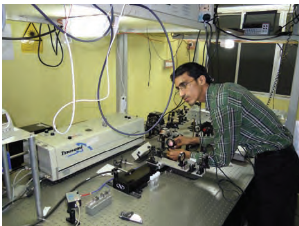
A PhD student is working on time-resolved spectroscopy setup using femtosecond laser system in the laboratory
