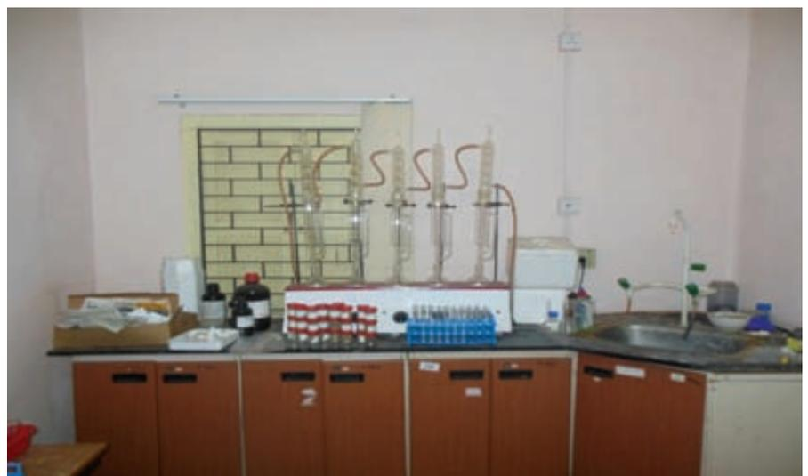
*Reflux set up for Nitrogen Estimation via Kjeldhal setup*
