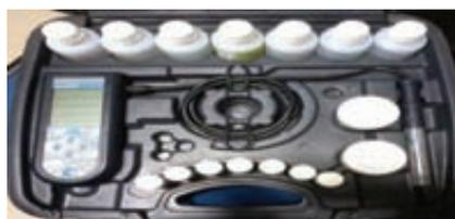
*Instrument for measuring pH, Oxidation/Reduction potential and Electrical conductivity*
