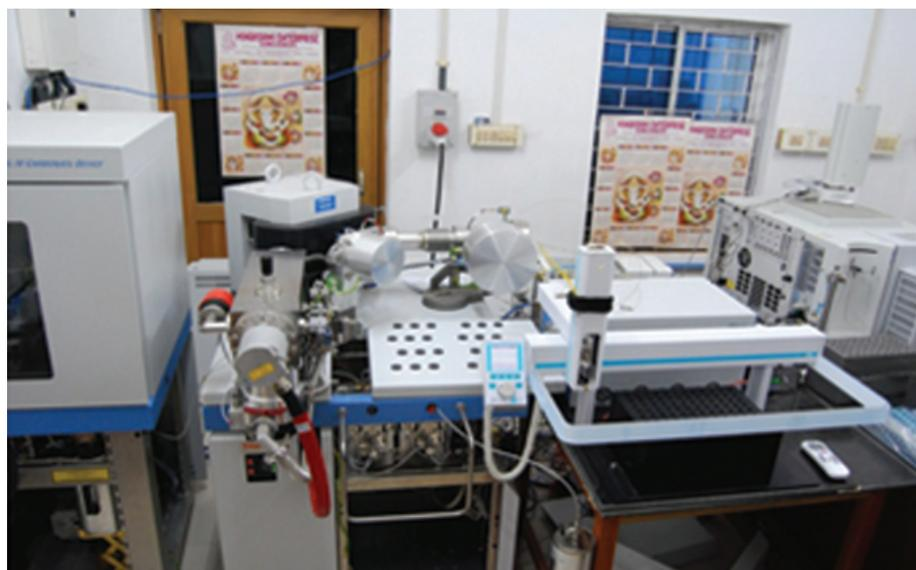
*MAT 253 with Gas Bench II; Gas bench is for water sample processing*
