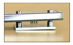
It consists of 4 collinear, equally spaced (2mm) and individually spring loaded probes mounted on a PCB strip. Two outer probes for supplying the constant current to the sample and two inner probes for measuring the voltage developed across these probes. This eliminate the error due to contact resistance which is particularly serious in semiconductors. A platform is also provided for placing the sample and mounting the Four Probes on It.
