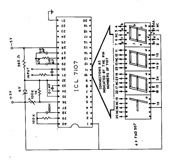
CIRCUIT DIAGRAM OF DIGITAL PANEL METER
