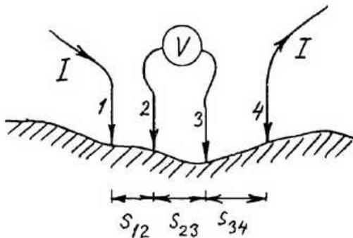
In practice, the contacts are produced by four probes with parallel movements as indicated. The resistivity is :
