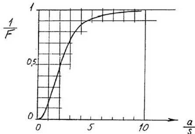
Geometric factor for infinitely long bar of quadratic cross section.
