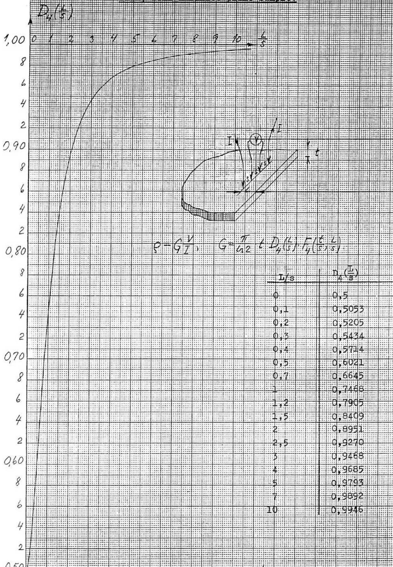
thin, semi-infinite plane sample.
