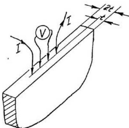
In example 2, section A.3, we showed that this configuration has the same geometric factor as has an infinite slice of thickness  $t$ , which is treated in section D.1 (thick sample) and section D.2 (thin sample).
