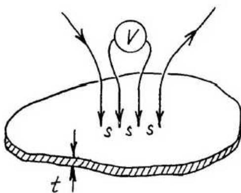
When the sample is thin, it is more convenient to write the resistivity in the form given by Smits ( $\epsilon$ ) :
