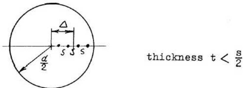
The geometric factor for the case, when the probes are lying on a diameter, but displaced from the center of the slice, has been calculated by Logan (i), and tabulated in detail by Swartzendruber (h).
