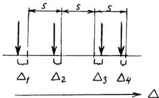
Probe displacements from equal distances.
