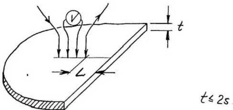
When the sample is thin, it is convenient to express the resistivity as follows :
