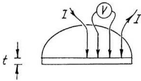
If we bisect the slice as shown, twice the voltage will develop between the inner probes for the same current.
