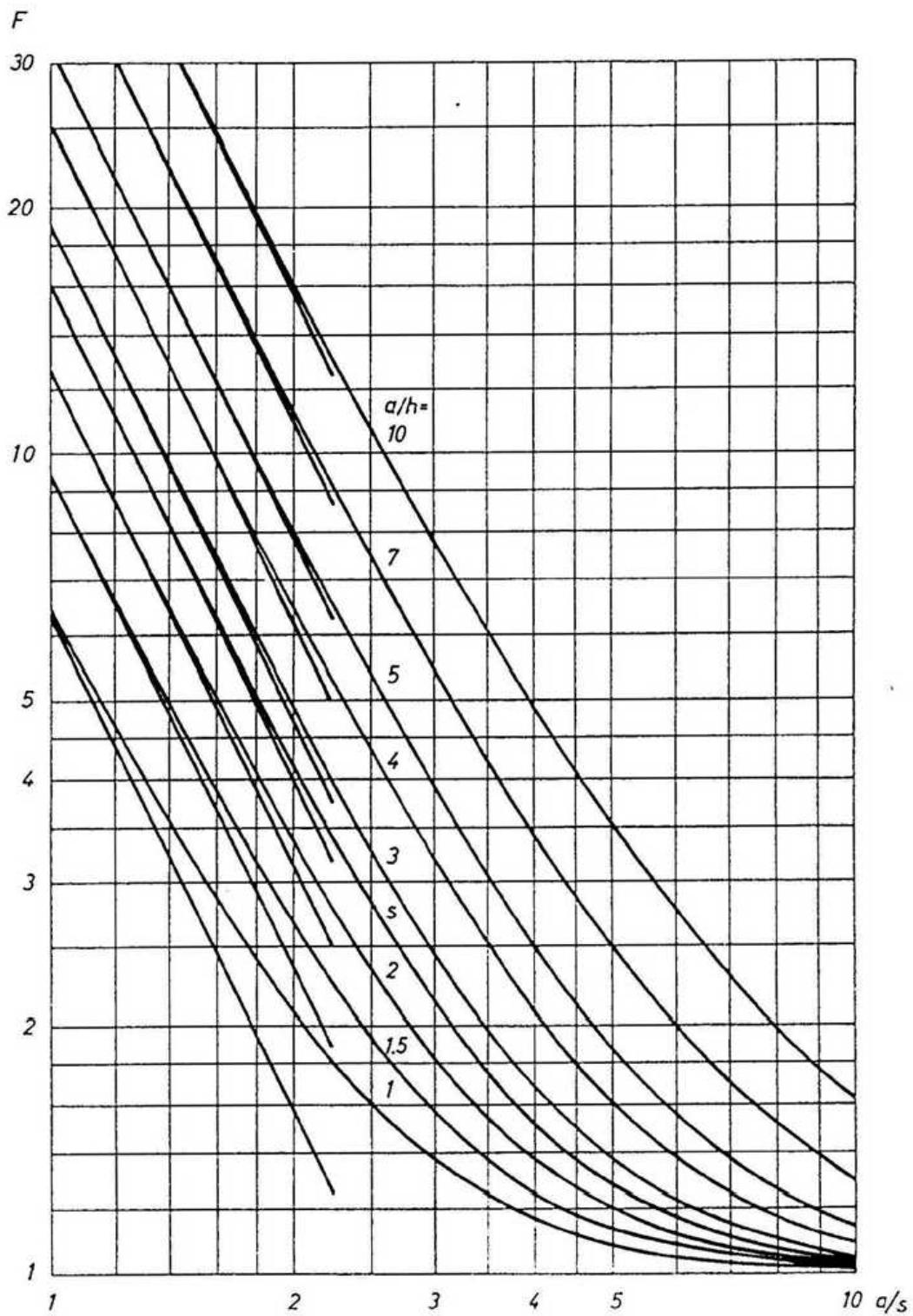
Fig. 2. The correction factor for an infinite bar of rectangular cross-section  $a \times h$  and for an infinite bar of semi-circular cross-section (indicated by an  $s$ ). The straight lines correspond to a homogeneous current distribution. The geometrical arrangements are shown in fig. 1 and fig. 4 respectively.
