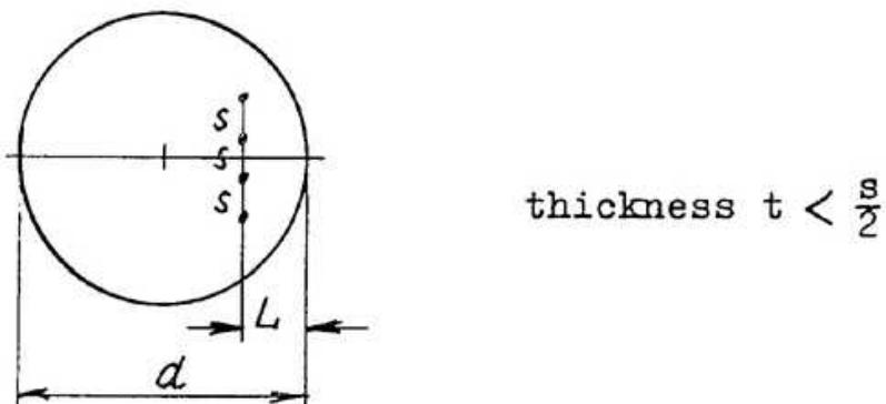
This special case of section I.3. is separately treated because of the common practice of specifying the resistivity of a slice by the values found in the center and at a specified distance from the edge.
