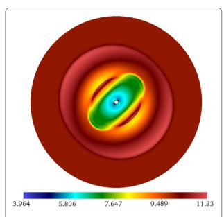
**Figure 17** Magnitude of the magnetic field from the solution to the blast wave problem at t = 0.07. A linear color scale is used
