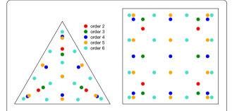
**Figure 8** Quadrature points on t-faces (left) and r-faces (right) of the prism. Three and four points are used to integrate a quadratic function exactly on t-faces and r-faces, respectively, four and six for cubic, six and nine for quartic, seven and twelve for quintic, and twelve and sixteen for sextic functions. The four point rule is not used on t-faces; instead the six point rule is used for third degree polynomials
