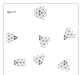
**Figure 10** Stencils of one selected face at division four near a penta-corner. Shown are the central stencil (top), the forward stencils (middle row) and the backward stencils (bottom row). The principal face is drawn with thick lines. Because of the penta-corner to the right of the principal face, some of the stencils have a different shape
