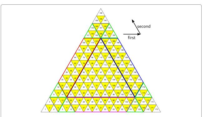
**Figure 3** A single sector of the mesh. In this example the face division is equal to the sector division plus three. The black arrows show the directions of the first and second TAS coordinates. Two layers of ghost faces are visible. The three trapezoidal and nine small triangular pieces marked with different border colors are the areas subject to boundary exchange with neighboring blocks
