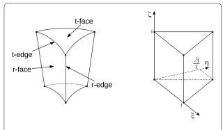
**Figure 5** A computational zone (left) and the reference element (right). The reference shape is a right equilateral triangular prism which is mapped into the frustum in physical space
