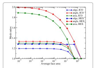
**Figure 2** Uniformity measures of the icosahedral mesh (triangles) and the hexahedral mesh (squares) for division 0–8 (former) and 0–9 (latter). Blue lines show edge ratios, red angle ratios, and green area ratios. The icosahedral TGM is measurably more uniform than the gnomonic cube sphere
