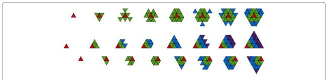
**Figure 9** Stencil shapes in the plane. The top, middle, and bottom rows show the central, forward-biased, and backward-biased stencils, respectively. The principal zone is shown in red. Green, blue, and purple colors represent first, second, and third von Neumann neighbors of the principal zone, respectively
