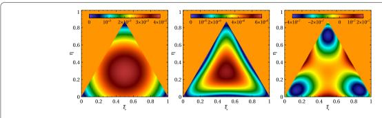
**Figure 7** Linear (left), quadratic (center), and cubic (right) mapping accuracy. Shown is the distance between the mapped surface and the perfect sphere computed for an equilateral triangle with a circumcircle radius of 5°
