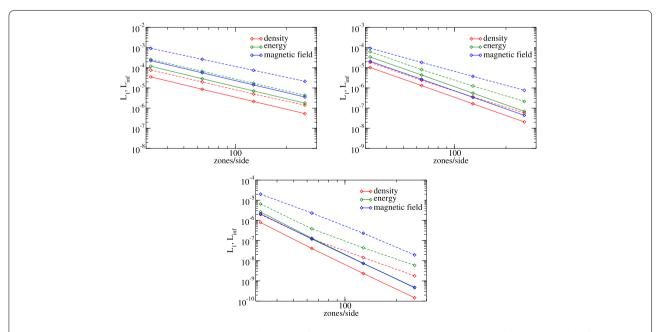
Figure 15  $L_1$  (solid lines) and  $L_\infty$  (dashed lines) norms of the error of density, total energy, and the x component of the magnetic field for the manufactured solution on division 4–7 TGM. The three panels correspond to second through fourth order schemes
