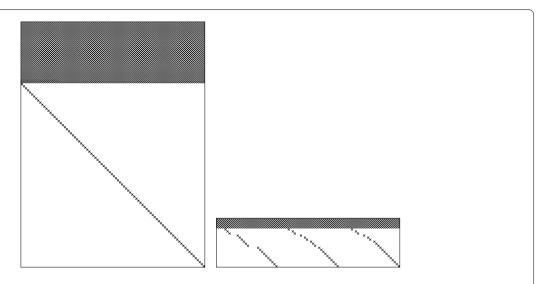
Figure 11 Matrix structure for divergence-free reconstruction. The left panel shows the nonzero elements (marked with x's) of the least squares matrix and the right panel shows the same for the constraint matrix for fourth order reconstruction. The corresponding KKT matrix is  $114 \times 114$
