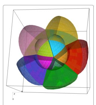
**Figure 12** Cutout view of the mesh showing ten blocks out of 20 (the smallest number of blocks on this mesh, consisting of a single slab and 20 division 0 sectors). Each block is shaded using a unique color
