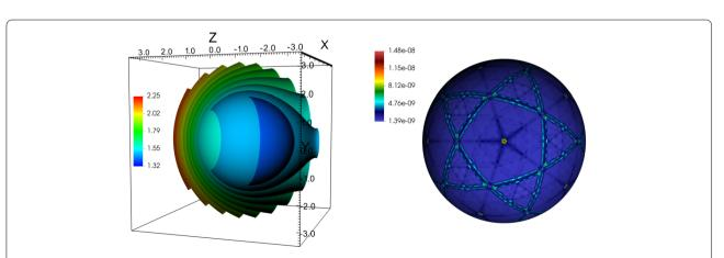
Figure 16 Left: velocity magnitude isosurfaces from the manufactured solution problem. The solution has a resemblance to an interaction between a stellar wind an a uniform flow. A fourth order scheme was used on division 6 mesh with 64 radial shells. Right: density error distribution in a spherical layer at r = 2.75
