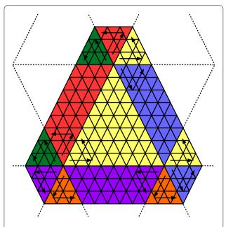
**Figure 13** Neighbor arrangement around a block. The pairs of arrows indicate the directions of the first and the second TAS coordinates, respectively. The different rotations of the TAS are shown with different color shading
