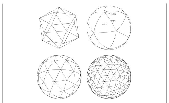
Figure 1 Recursive icosahedral mesh generation. Shown are the inscribed icosahedron (top left) and the division 0 (top right), 1 (bottom left), and 2 (bottom right) triangular tesselations. The edges of the tesselation are repeatedly bisected until a desired level of refinement is reached
